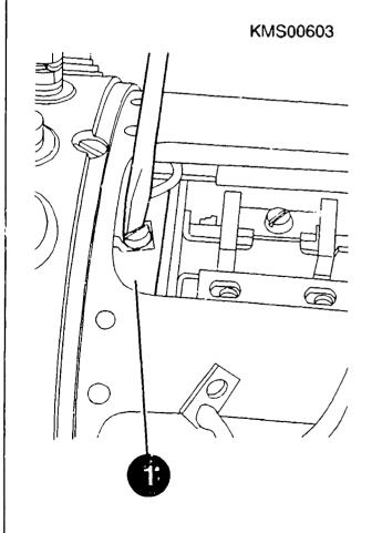
Completely disassemble connection term. 50 (1).
